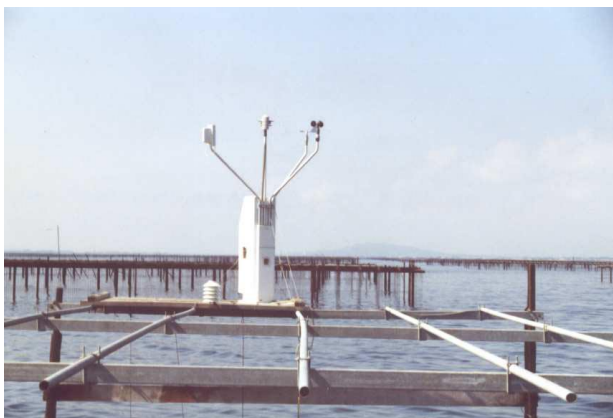
GSM water-level ENERCO 408 weather station (Thau pond) Ecosystèmes lagunaires – University of Montpellier II / CNRS
