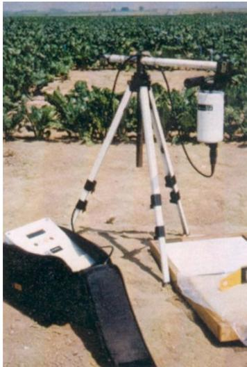
The CE 313-2 version is equipped with two detectors : one silicon detector for measurements in the 350-1100 nm band and one InGaAs detector for measurement in the infrared range from 1100 to 2500 nm. Up to nine user adjustable filter can be mounted on the instrument.
