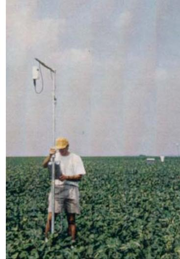
The CE313-1 version has one silicon detector for measurements in the 350-1100 nm range and can be equipped with up to 9 user adjustable filters.
